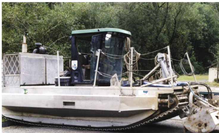
Amphibious tractor equipped with WeedSeeker® selective spray system in Willapa Bay, Oregon.
