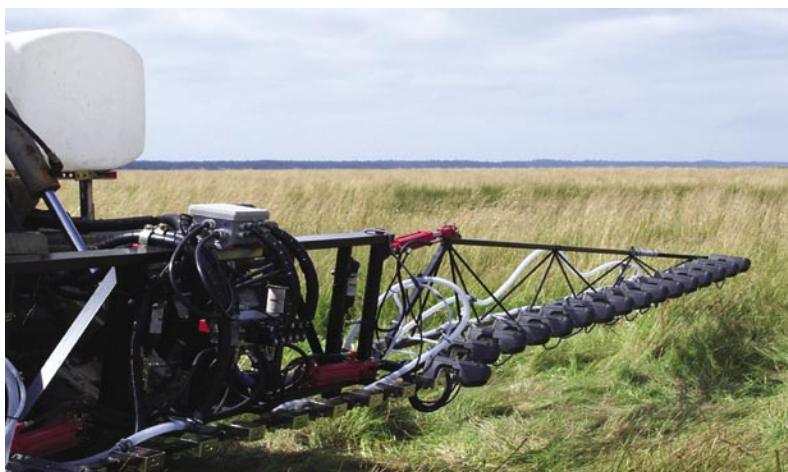
WeedSeeker® selective spray system mounted on the front boom.
